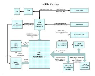
*Figure 3. – (e)film detailed block/functional diagram*
