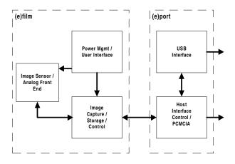
Figure 2. Functional Block Diagram of (e)film and (e)port
